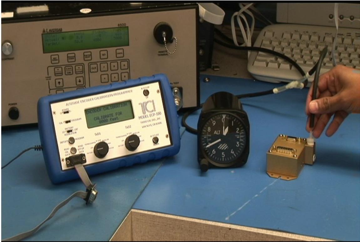
I'll begin by connecting the static pressure source to the encoder and the altimeter.
