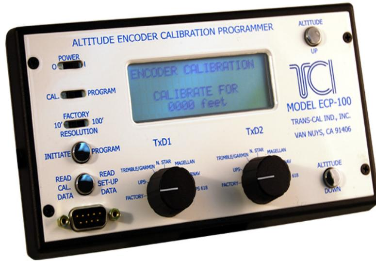
Using the ECP-100 an avionics technician may enter a digital correction to the altitude encoder's error curve in 1000' increments.
