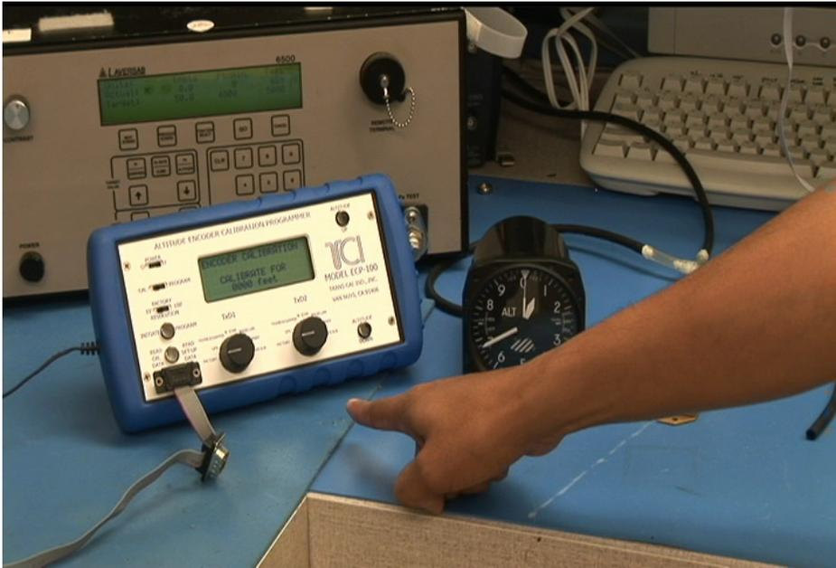
Our set-up consists of an altitude encoder with a serial port,
