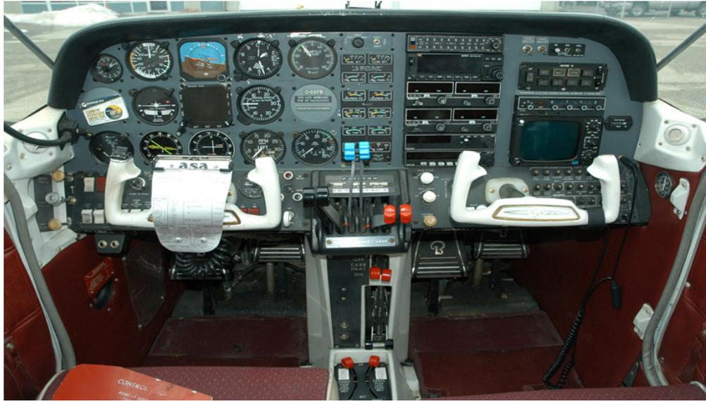
When an altitude encoder is installed in an aircraft to be used as the transponder's source of "Mode C" information it must "match" or correspond to the aircraft's primary flight altimeter within  $\pm 125$  feet, as required by FAR 91.217 and 91.411.
