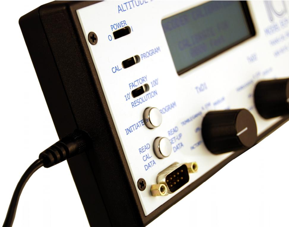
Even though we are doing this procedure on the bench it could easily be done in the aircraft. The ECP-100 may be powered through it's internal 9 volt battery or, as we are doing here, through an AC adapter.
