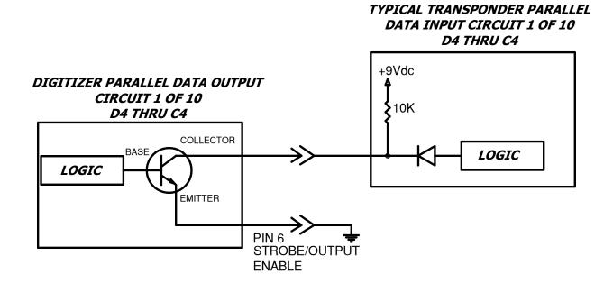
3. Why do altitude encoding errors occur when connecting a second or third device to the altitude encoder, but not when only one device is connected?
